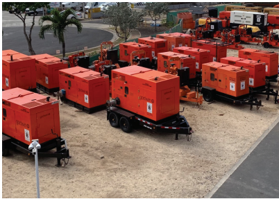
Dri-Prime Pumps for Sewer Bypassing & Dewatering
